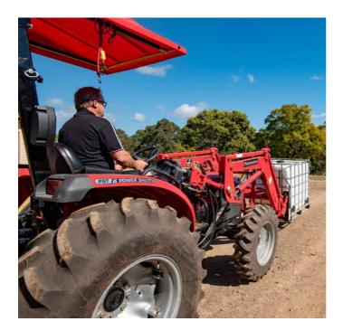
**HEAVY DUTY FRONT AXLE** The heavy-duty front axle ensures maximum reliability in loader and field operations. The bevel gear front axle with a responsive hydrostatic steering provides a tight steering angle, so getting in and out of confined areas is easy.
